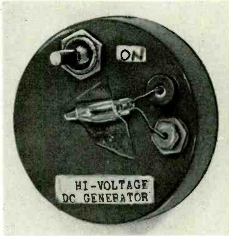
Front view—neon lamp acts as indicator.
