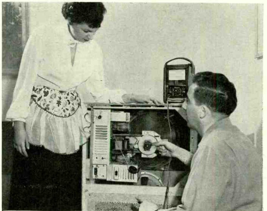
"... I reasoned it was the filament in the picture tube or the 6W6 damper."
